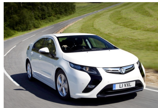
Figure 1. The Vauxhall Ampera is an example of a 'plug-in hybrid', scheduled to enter the UK market in 2012. Its battery can store 16 kWh which gives it a pure electric range of 80 km. It also contains a petrol-electric generator to extend its range. Photo © Vauxhall.
