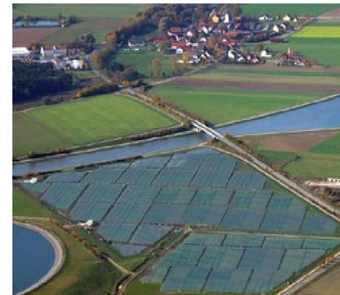
Figure 2. The peak power delivered by this 25 000 m 2 solar photovoltaic farm in Muhlhausen, Bavaria is about 6.3 MW. The average is 0.7 MW, so the average power per unit area is 5 W/m 2 .
