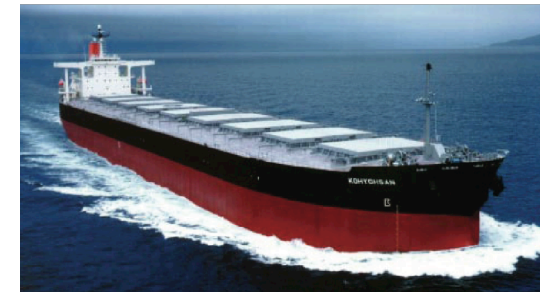
Figure 1. The Kohyohsan, a ship built with an 'axe bow' that reduces the energy lost in waves, reducing fuel consumption by up to 6%. Source: IMO.
